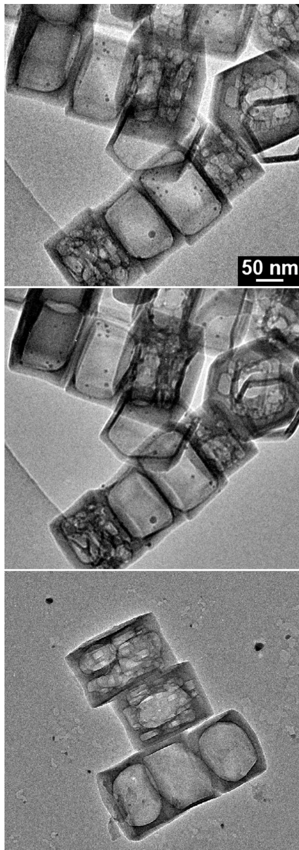
Fig. 2: a): Assembly of silica cages containing Ag NPs at 20^\circ\text{C} under high vacuum; b): same area at 700^\circ\text{C} under high vacuum: the Ag NPs have grown but are mostly still inside the silica-cages; c): other area at 450^\circ\text{C} under 2 \cdot 10^{-2} mbar of \text{O}_2 flow: note that all Ag NPs are out of the cages on the carbon supporting film, contrarily to b).
