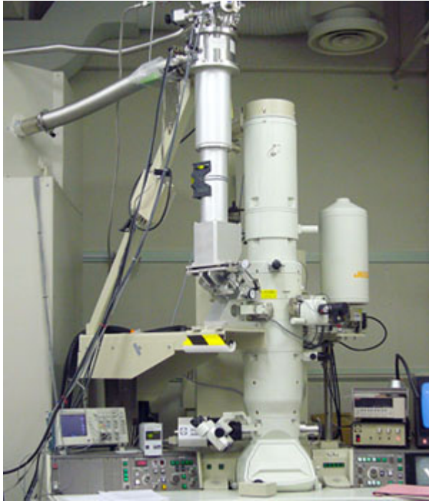
Fig. 1: Figure 1. Transition-Edge Sensor type microcalorimeter EDS mounted on a TEM.
