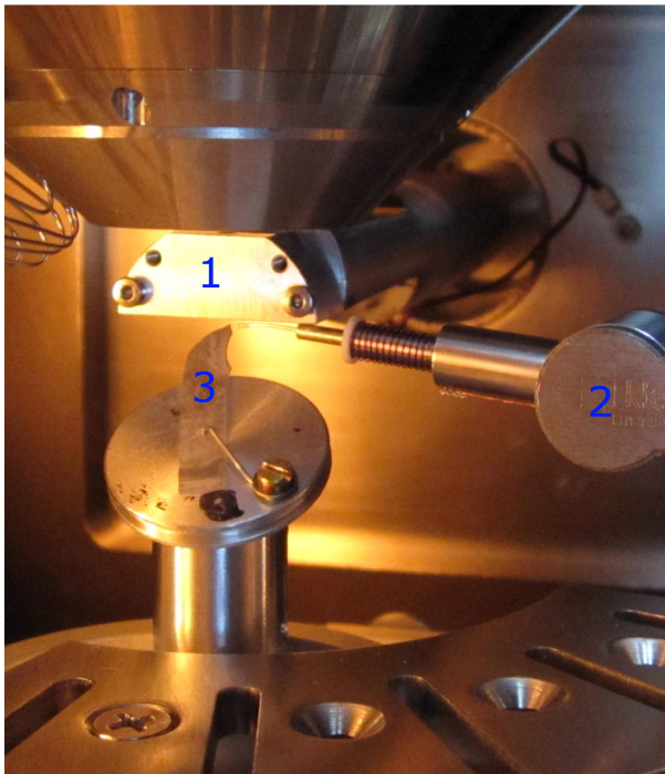
Fig. 2: Photograph of the CL-SEM chamber showing the arrangement of the parabolic mirror (1) for light collection, the micromanipulator (2) and sample (3) tilted by 30^\circ . The sample is contacted inside the focal point of the optical collection system by a tungsten probe tip attached to the micromanipulator.
