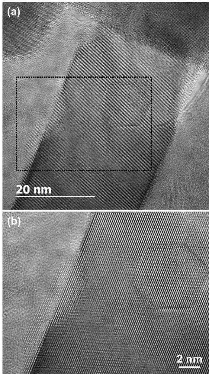
Fig. 1: (a)  $\text{TiO}_2$  substrate classically used in catalytic reactions with nanoalloys imaged under 1 bar pressure of  $\text{O}_2$  and at  $1000^\circ\text{C}$  (with a JEOL ARM 200F cold FEG microscope equipped with an aberration corrector of the objective lens). (b) Enlargement of the rectangular area in dotted line of (a).
