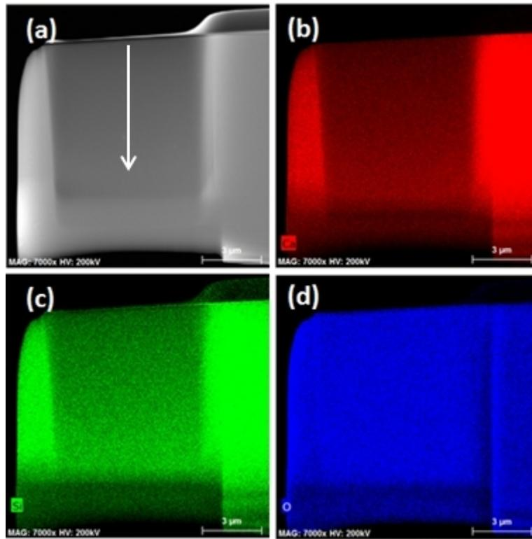
Fig. 1: HAADF-STEM image of wollastinite recorded on a Tecnai-OSIRIS (a) and EDX elemental maps of Ca (b), Si (c) and O (d) using the Super-X detector.
