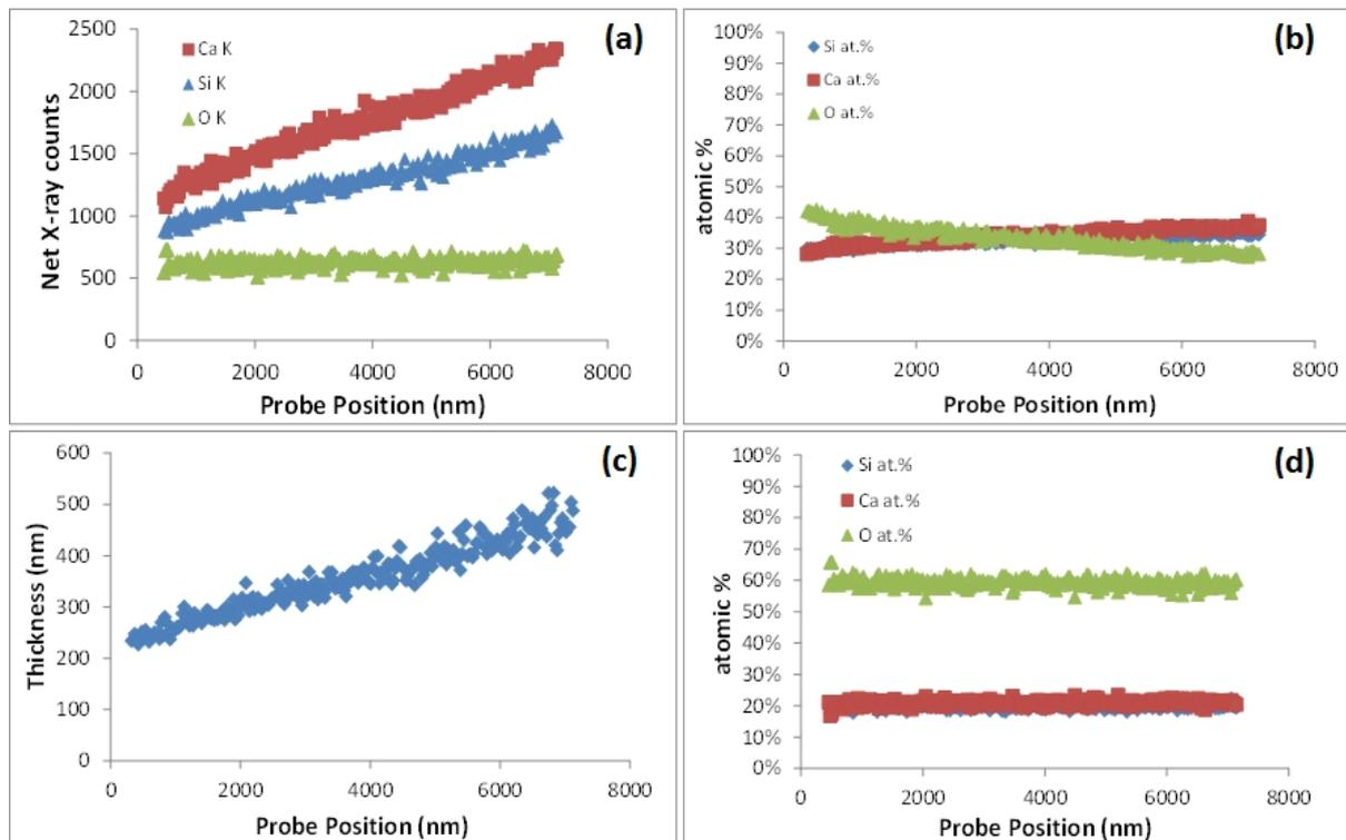
Fig. 2: EDX Line scan extracted from the site marked with an arrow (a). EDX quantification using the k-factor method (b). Thickness measurement obtained by EDX analysis (c) and EDX quantification in atomic percentage using the  $\zeta$  (zeta)-factor (d).
