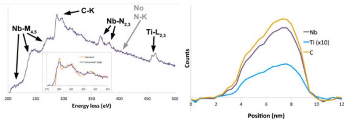
Fig. 2: The background subtracted spectrum of the core loss EEL spectrum from the central region of the NbC precipitate, and profiles of the integrated counts in a horizontal line across the centre of the precipitate. Ti counts have been multiplied by a factor of 10 for the purpose of this graph.
