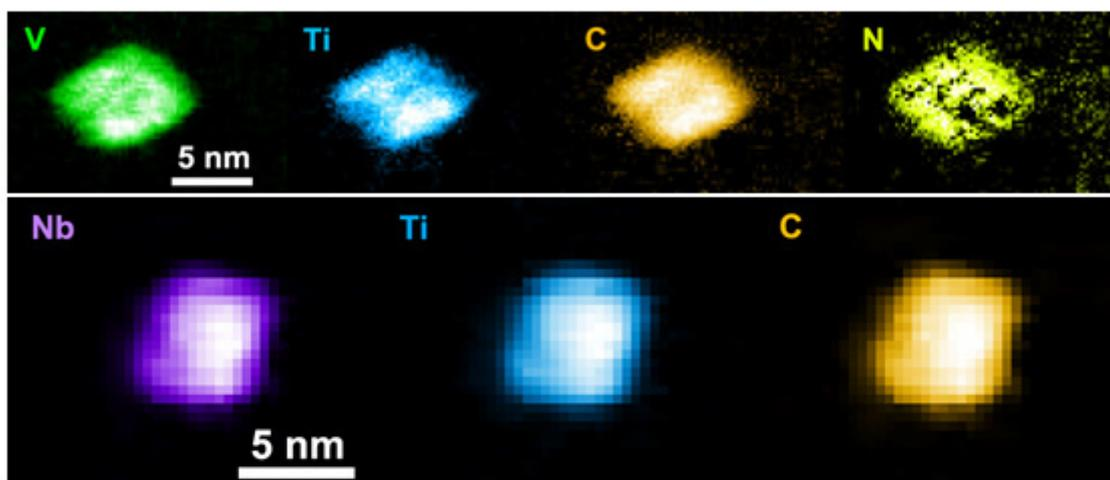
Fig. 1: Qualitative maps processed from spectrum images of vanadium carbide and niobium carbide precipitates, both from steels isothermally treated at 900°C for a fixed time of 100s followed by quenching. The vanadium precipitate after the background subtraction reveals small traces of N.
